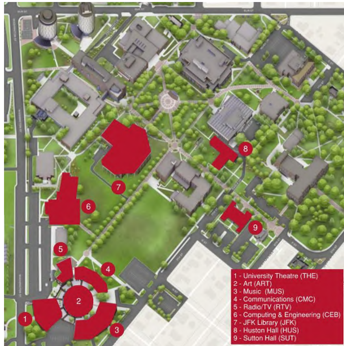
Figure 1: Buildings Connecting to First Geothermal Node
