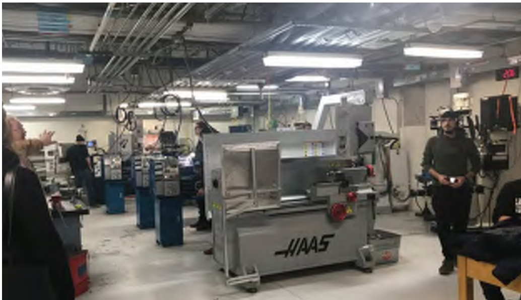
EWU MENT teaching lab facilities with substandard overhead clearances in the CEB basement
