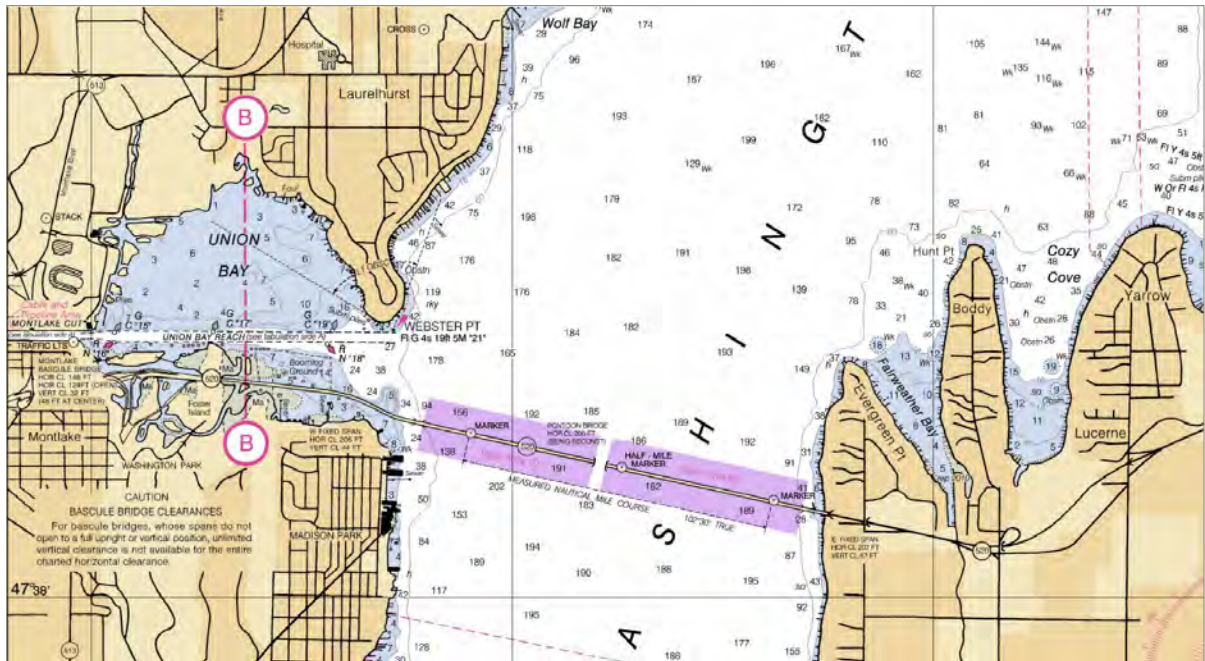
Exhibit 5-2: Bathymetry of Lake Washington in the Vicinity of the University of Washington and the Ship Channel (Soundings in Feet Relative to Local Mean Lower Low Water) 9
