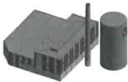
1.0 Million Gallon Thermal Storage Tank Perspective View
